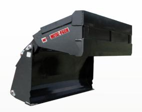
The bucket is intended for picking, loading and transporting various materials. The accessory facilitates earth work and reloading of scooped material. The device can also carry the load at short driving distances. The accessory is intended for agriculture, forestry and community services. The Hardox wear-resistant shares assure long life of the machine. Mounted mobile section of the bucket, operated with two hydraulic cylinders, allows a wide opening angle.
