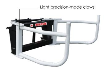
The bale grip is intended for transporting bales of straw, hay and silage. Equipped with one double-action cylinder and a special strut to guarantee simultaneous opening and closing of both arms. The light structure of claws reduces the machine weight for better stability of the tractor. Durable powder-painting coat.
