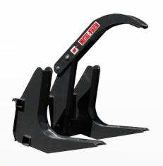
The KRAB timber clamp is mainly intended for forestry and saw mill applications. The device can swiftly pick timbers from storage, load them on transport vehicles, or simply transport them from one place to the other. The handled ltimber is pressed against the forks with a moving arm, operated by a hydraulic cylinder connected via quick-release couplings to the front loader's solenoid valve.
