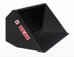
The bulk material bucket is a solid accessory available in the working width range from 1.4 m to 2.2 m. Its large capacity makes the accessory ideal for transporting light bulk materials, namely grain or fertilizers. The backwards-tapered shape facilitates scooping the material and filling the bucket fully. The share is made from wear resistant material. EURO mounting as standard. Durable powder-painting coat.
