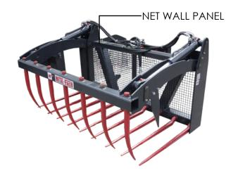
Manure grips are intended for transporting manure and maize, among others. The manure grip is mounted on the front loaders. Equipped with two cylinders. This model is available in three width sizes: 1.2 m, 1.5 m and 1.8 m. The load capacity depends on the size version and ranges from 500 to 800 kg. The back wall panel of this new Metal-Fach Type Z model is made from a specially designed net.
