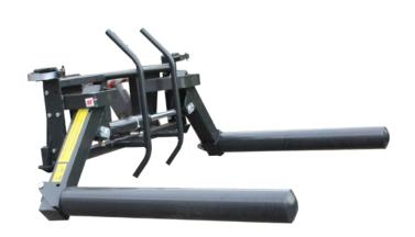
Multifunctional grip is intended for picking, transporting and loading bales on trailers. Its multipurpose design allows bale transporting by gripping or piercing with forks as well as easy loading and unloading of silage bales. The installed guards facilitate loading of wrapped bales without piercing or ripping the film. The grip can easily hold up to three bales of hay or silage. The fork guards are easy to disassemble. Bales can be grabbed horizontally or vertically.
